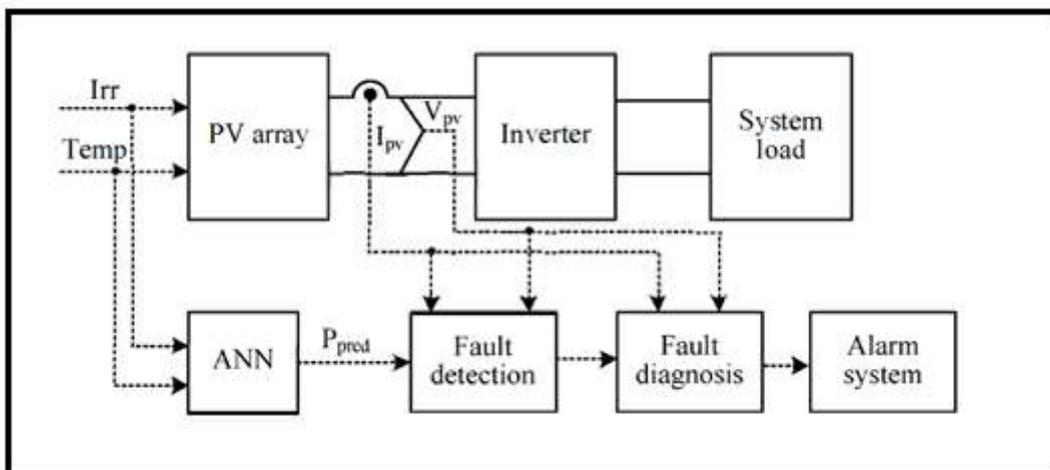
Fig.3. The PV system with fault detection and diagnosis [4]
