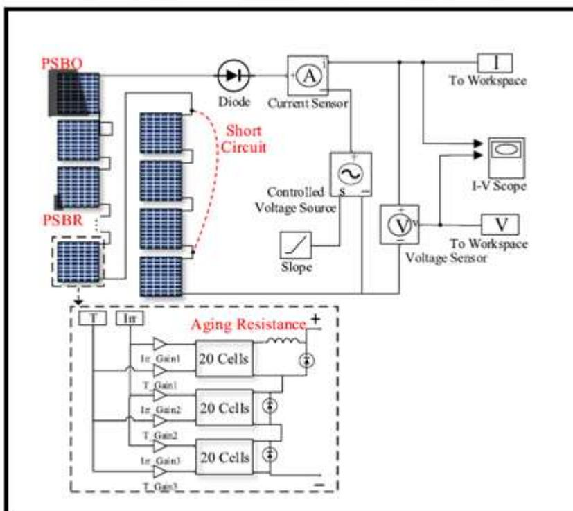
Fig.8. I-V testing circuit and PV module modeling via MATLAB/Simulink [11]
