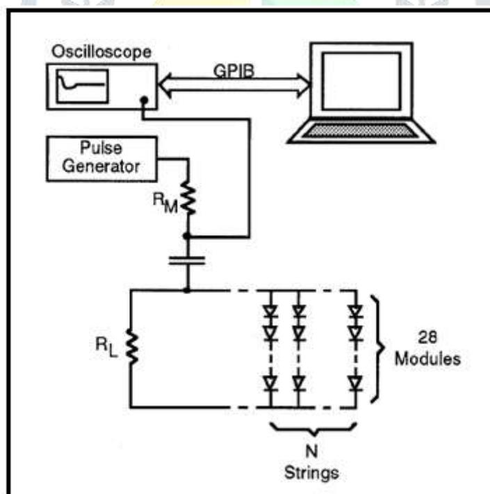
**Fig.2.** Step excitation voltage based approach [2]
