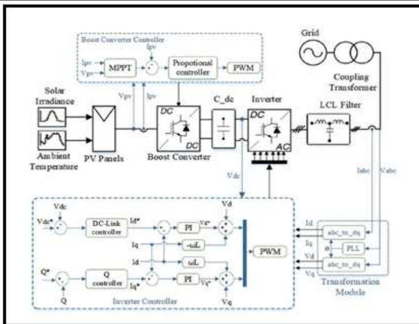
Fig.7. Control structure of the GCPV system [10]
