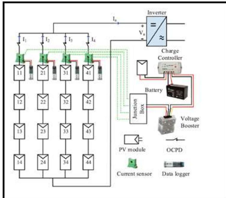
Fig.5. Solar PV fault analysis system model set up [6]
