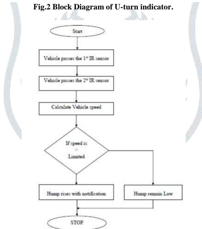
**Fig.3 Flowchart of speed breaker system.**
