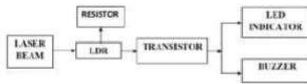
**Fig.2 Block Diagram of U-turn indicator.**
