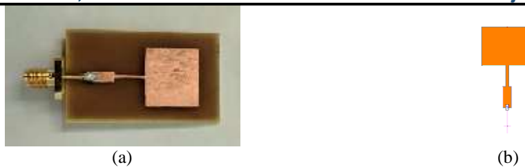
Fig. 1 (a) Top view of Microstrip patch antenna for single element, (b) Geometry of microstrip patch antenna for single element
