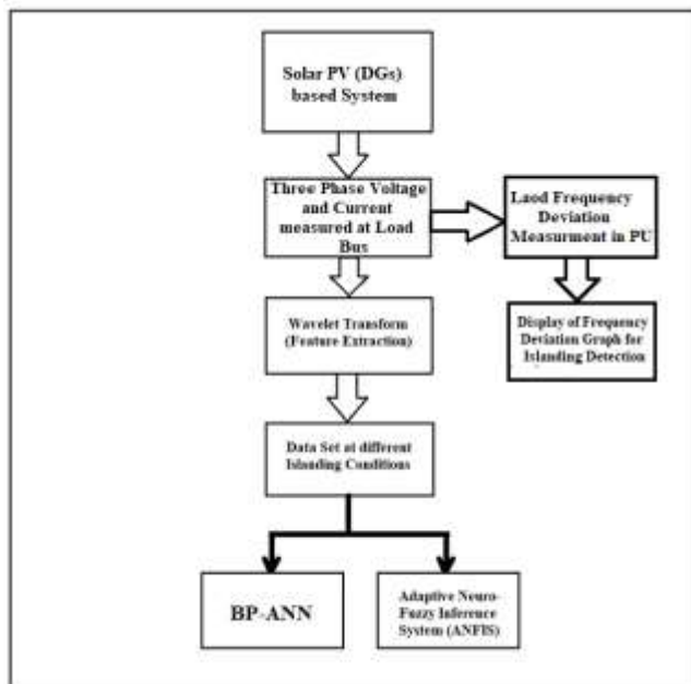
Fig.5. Flow block diagram of proposed islanding detection techniques
