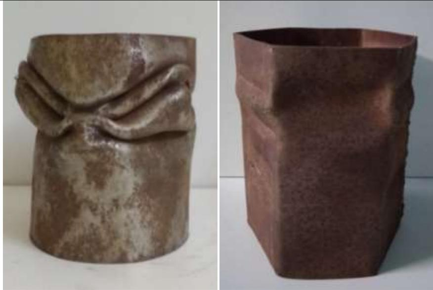
Fig. 4 Total Deformation of Circular and Hexagonal shape Crash Box Experimentally
