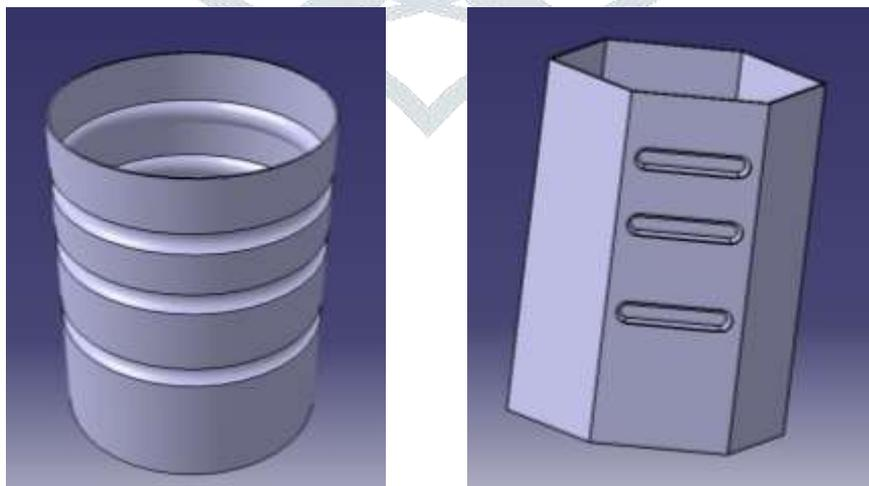
Fig.1 CAD Model of Circular and Hexagonal Shape Crash Box
