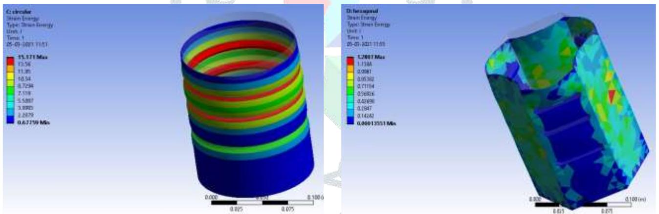
Fig. 3 Strain Energy of Circular and Hexagonal shape Crash Box
