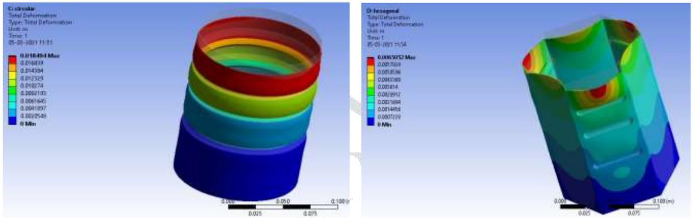
Fig. 2 Total Deformation of Circular and Hexagonal shape Crash Box
