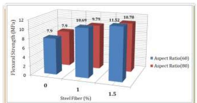
Fig -4: Flexural strength of concrete mixed with 10% metakaolin and hooked steel fiber of different aspect ratios.
