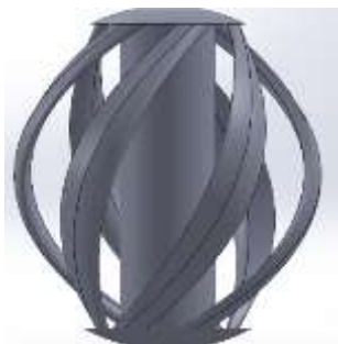
(a) CAD Model of Runner; (b) Assembled view of Runner and Pipe
