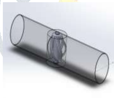
(a) CAD Model of Runner; (b) Assembled view of Runner and Pipe
