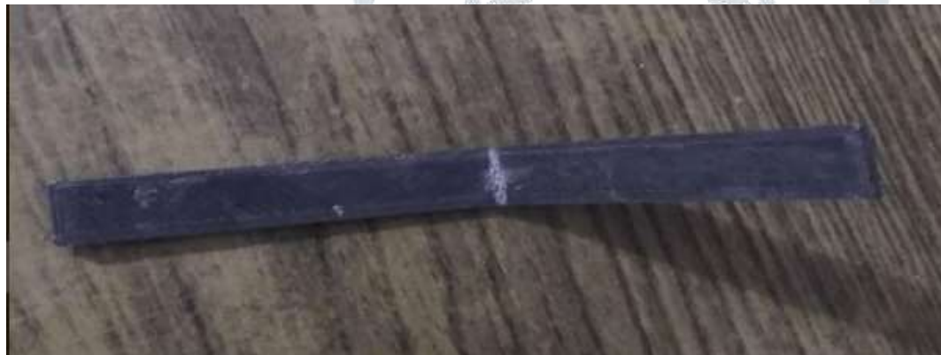
Figure: FLEXURAL SPECIMEN AFTER TESTING
