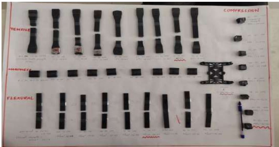
Figure: All Specimens After Testing
