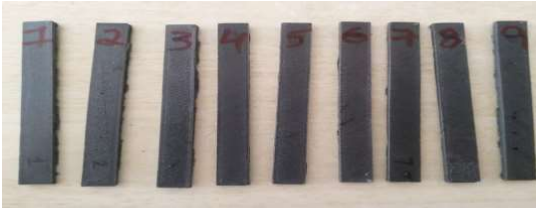
Figure: FLEXURAL SPECIMEN BEFORE TESTING
