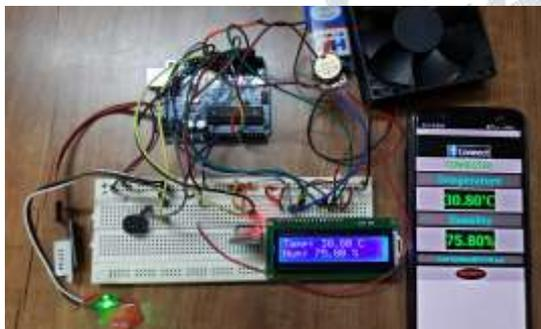
Fig. 9: System with readings on mobile application
