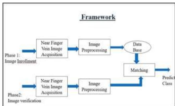
Fig. 1 Framework for finger vein system
