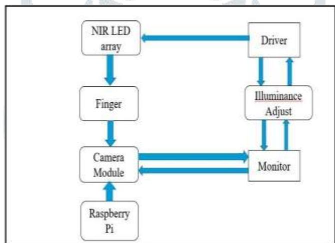
Fig. 2 Image acquisition module.
