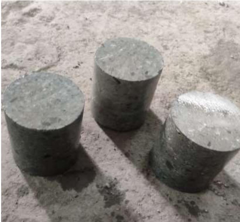
Fig 4 showing casted cores
