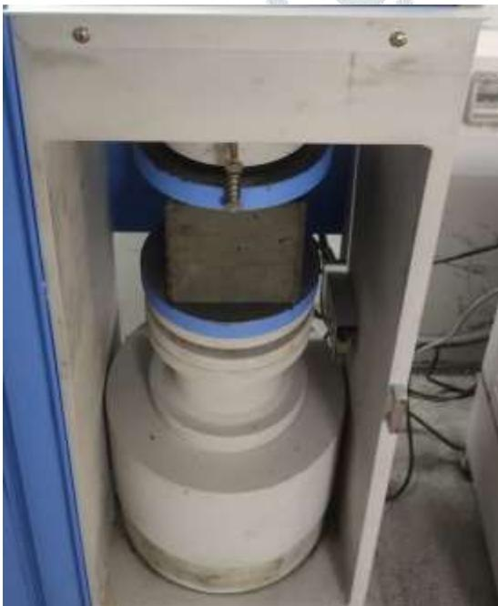
Fig 2 showing cube in compression testing machine
