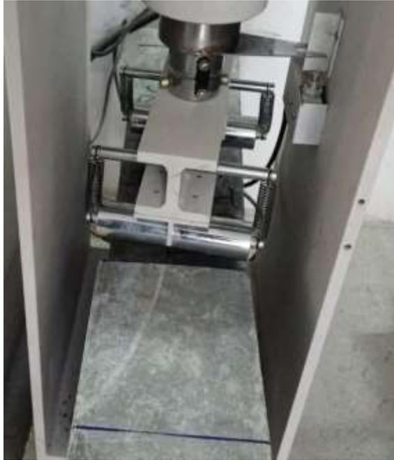
Fig 3 showing beam in the flexural testing machine
