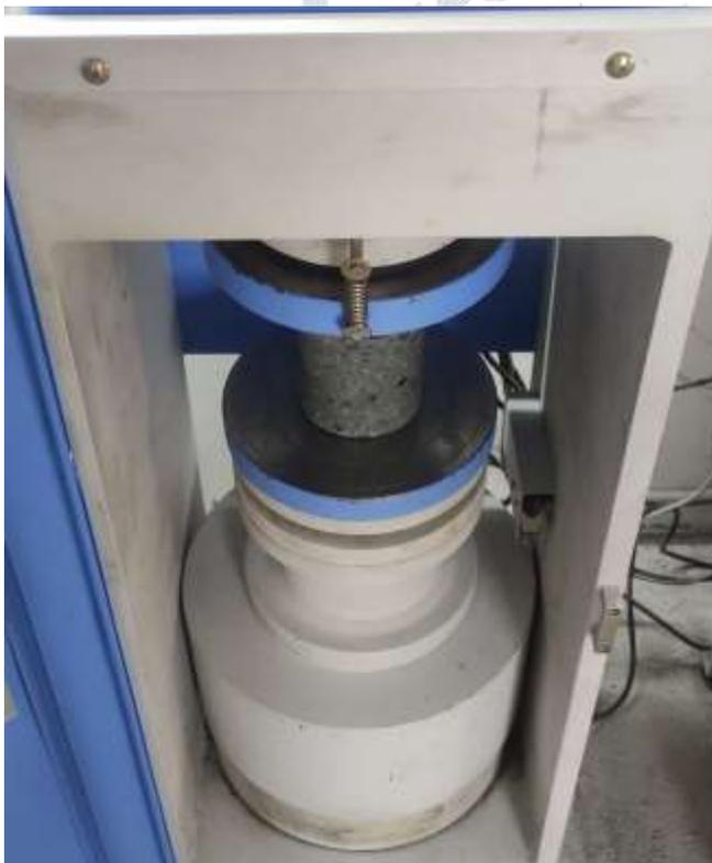
Fig 5 showing core in the compression testing machine
