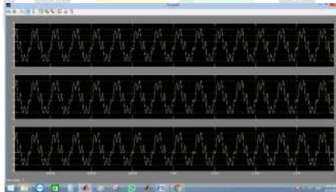
Fig 6: The primary current of the transformers.
