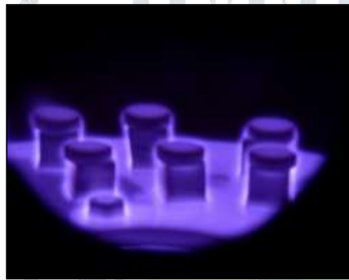
Figure 3- Thermal spray coating inside chamber
