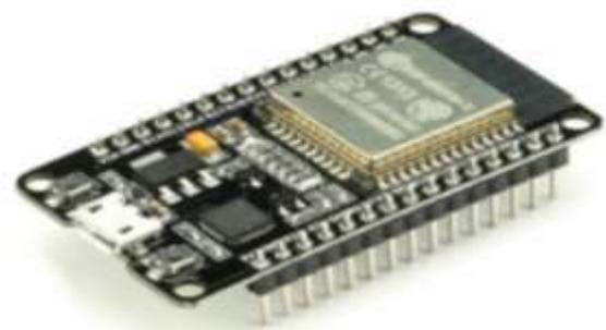
Figure 3.2: ESP32 Development Board with WiFi
