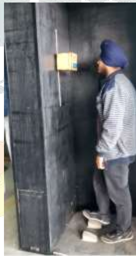
Person Adjusting the Sensor Unit according to his height using the foot pedals provided down there, So that the temperature sensor is pointing towards his forehead.
