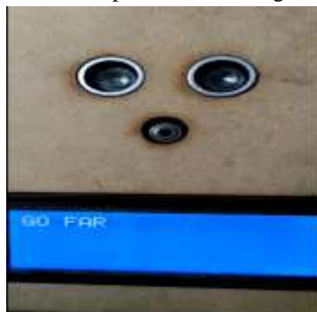
As the person is standing to close to the Sensor unit the LCD Display Shows “GO FAR”
