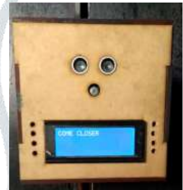
As the person is standing far from the Sensor unit the LCD Display Shows “COME CLOSER”
