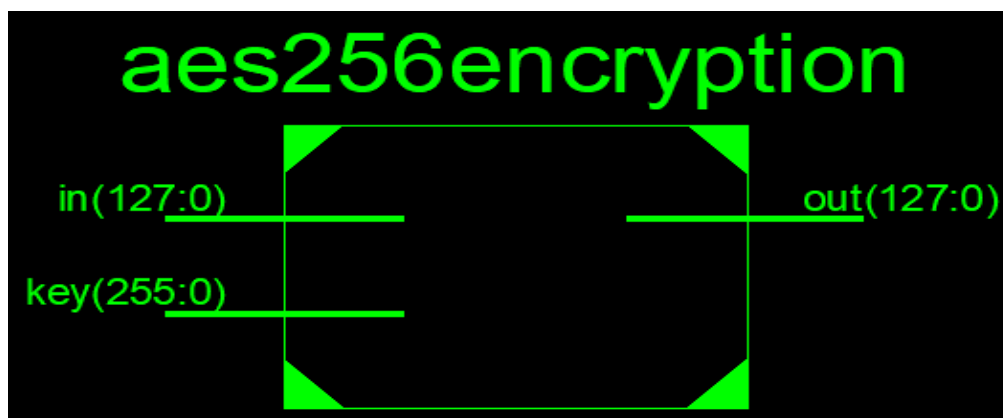
Figure 3: RTL Schematics of WiMax/IOT MAES
