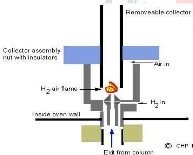
One of the major areas of application for the FID is in the analysis of hydrocarbons although it is also employed extensively for pharmaceutical analysis, pesticide analysis, forensic chemistry and essential oil analysis. Nevertheless, its major area of application is in the analytical laboratories of the hydrocarbon industry.
