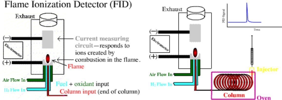
Hydrogen is mixed with the column eluent and burned at a small jet. Surrounding the flame is a cylindrical electrode and a relatively high voltage is applied between the jet and the electrode to collect the ions that are formed in the flame. The resulting current is amplified by a high impedance amplifier and the output fed to a data acquisition system or a potentiometric recorder.
