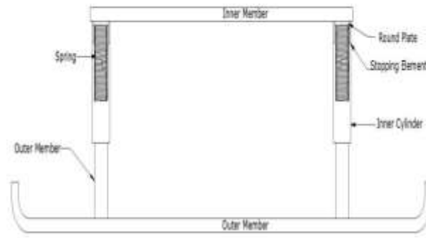
Fig:3 the proposed design of safety impact guard
