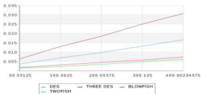
Fig. 8 : File size (in kb) [X axis] vs execution time (in s) [Y-axis] comparative graph for decryption using DES, 3DES, Blowfish and Twofish
