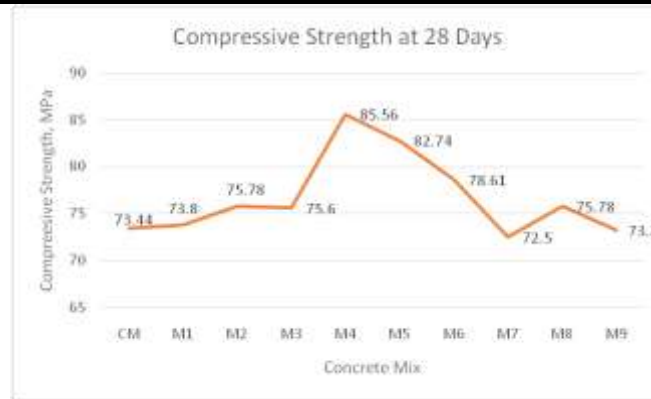
Figure 3. Compressive strength at 28 days.
