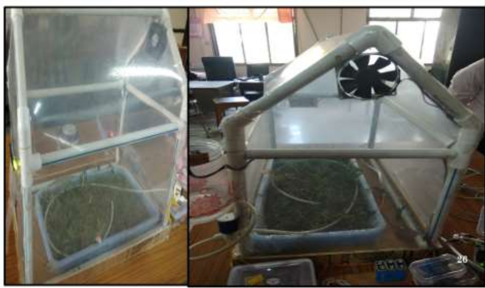
Figure 2: Hardware setup of IoT Based Climate monitoring and controlling system of GHS
