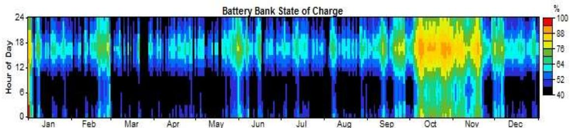
**Fig. 5.5** Battery state of charge
