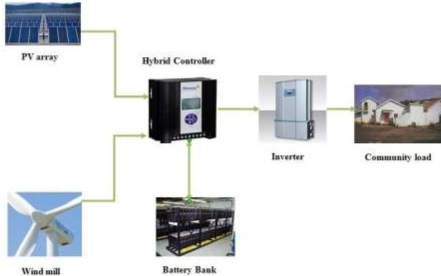
Fig. 4.1 PV-wind hybrid system
