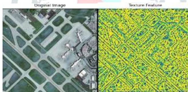
Figure 4. showing the texture features extracted from the image using LBP
