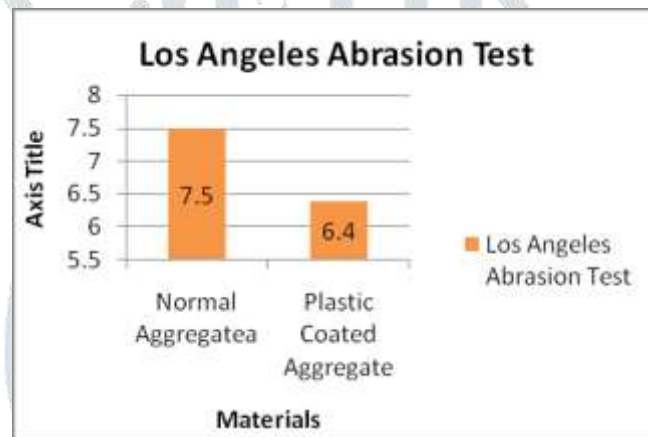
FIG 6 Aggregate abrasion value Test
