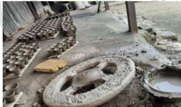
Plate 5: The traditional wheel to make mus cup and mud glass in the house of Lakhhi Pal of Kasba Mahaso
