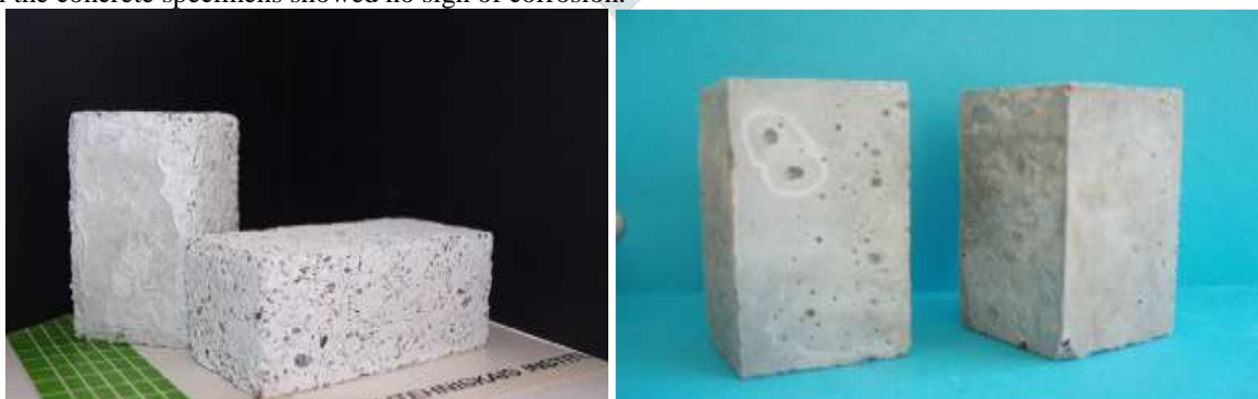
Fig. 2: Concrete with micro-silica after sulphate solution attack simulation in H 2 SO 4 (a); Na 2 SO 4 (b) for 200 days
