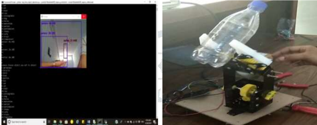
Fig8. (a) Capturing image (b) Picking and placing the object with a robotic arm
