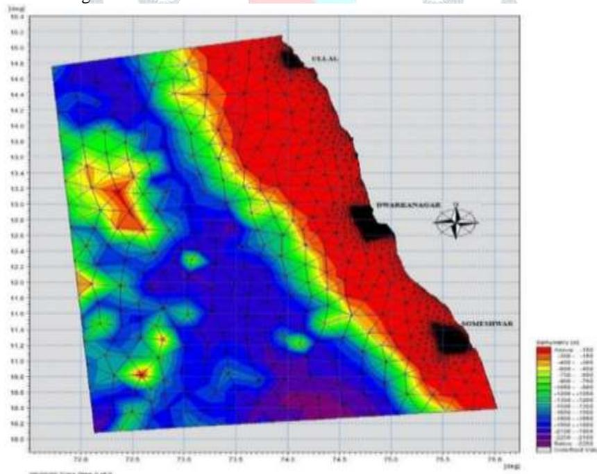
**Fig. 2:** Mesh Generated for entire bathymetry
