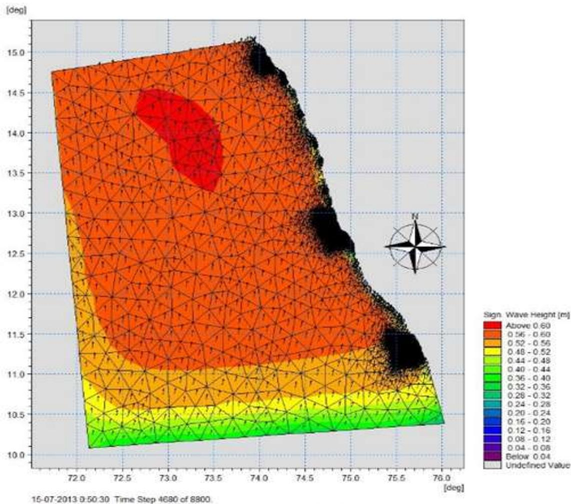
Fig. 6 Wave height and direction vectors in the region near Ullal
