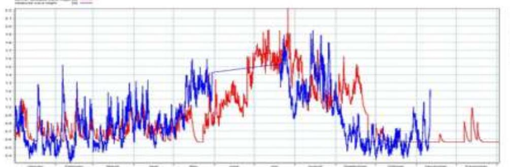
**Fig.4:** Comparison of measured and simulated significant wave height
