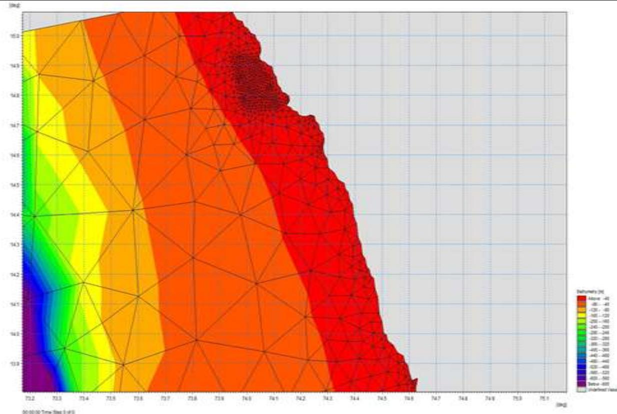
**Fig. 3** Mesh Generated Bathymetry near Ullal
