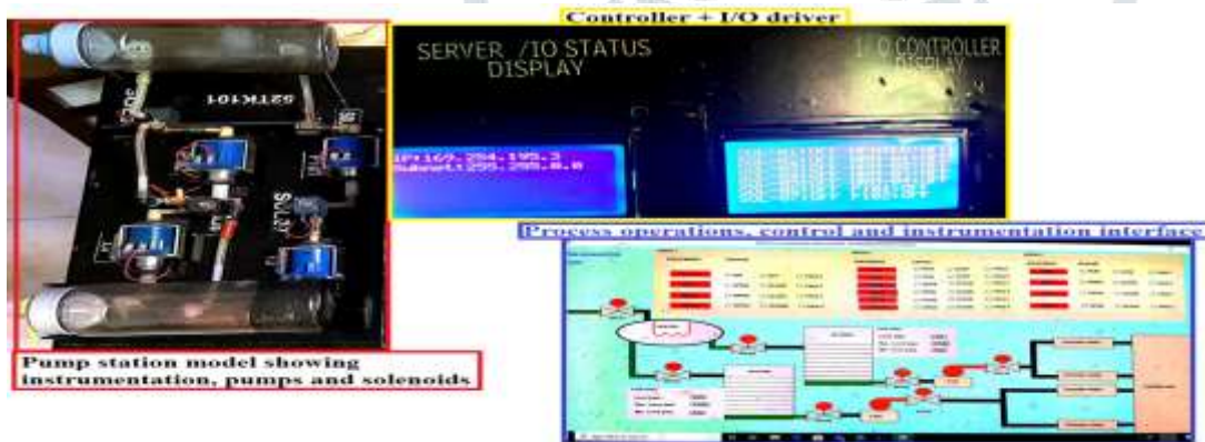
Fig.7. Integration of model, software and HiL (Controller).
