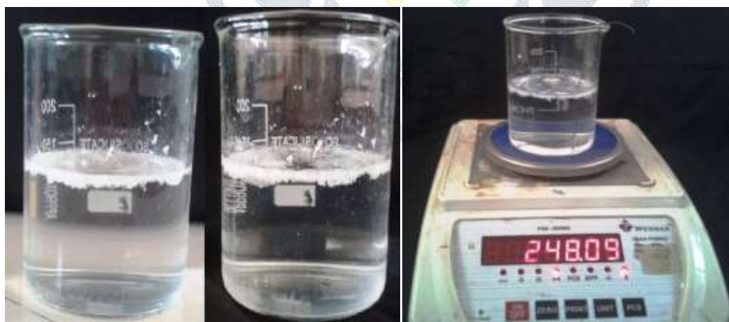
Fig 7: Formation of raft and Measurement of raft strength
