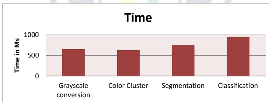
Figure 2 : Time required for single image processing with various function in stand alone system
