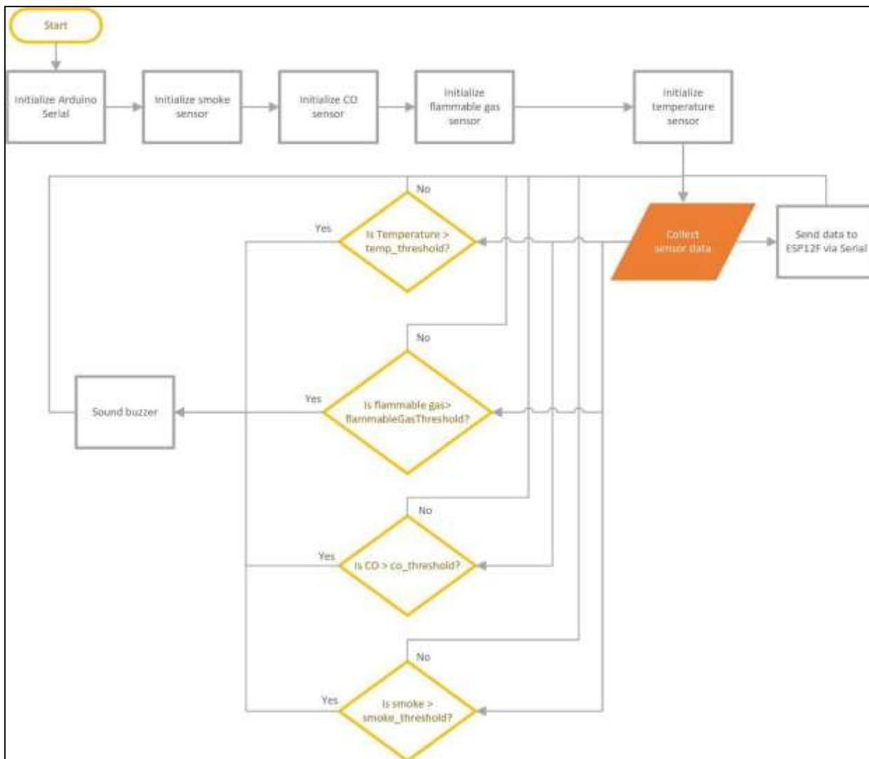
Figure.5: Flowchart for Sensor-Arduino Nano Interfacing
