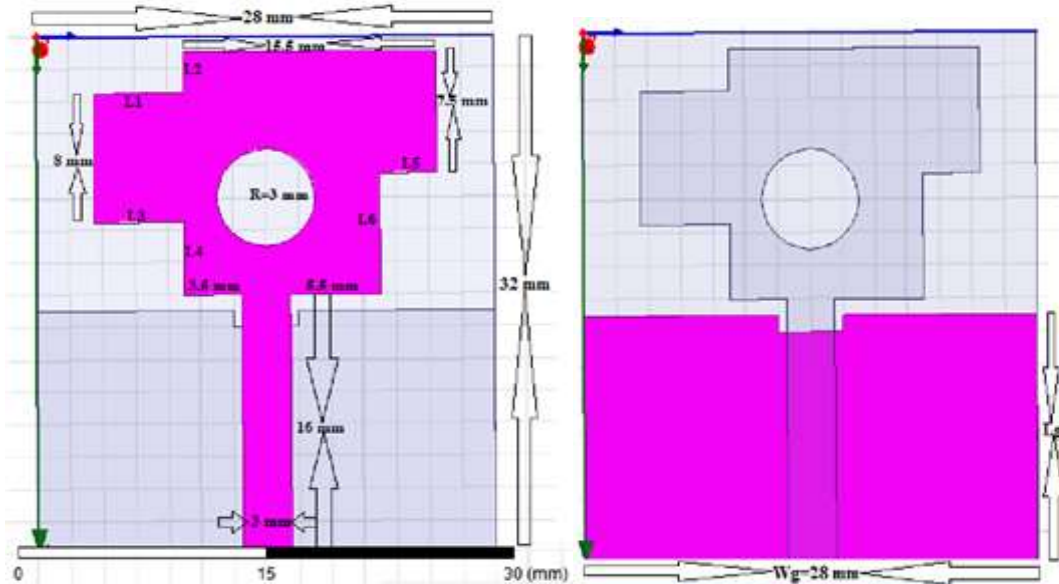
Figure 2 Patch view and Ground of the antenna
