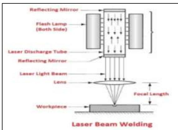
Figure 1: Laser Beam Welding
