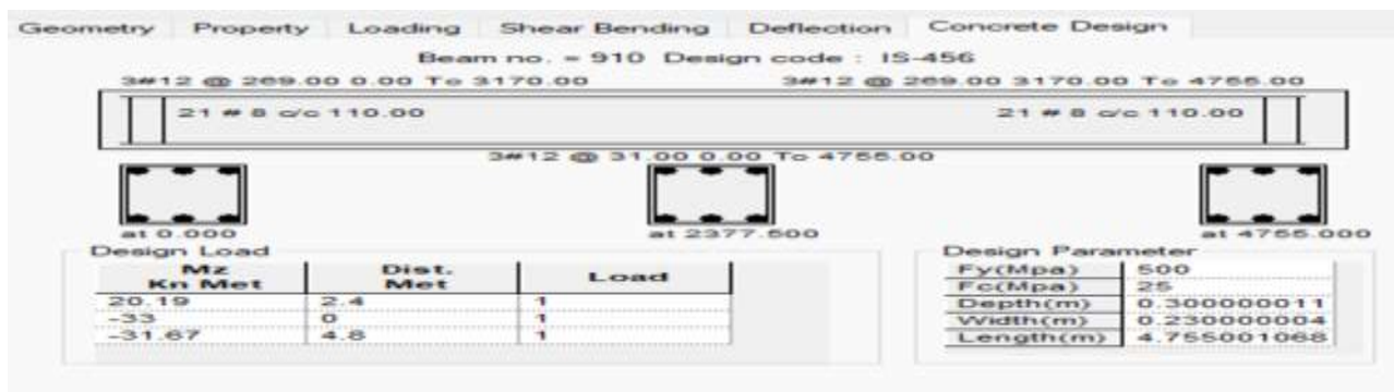
Fig-5: Reinforcement details of beam
