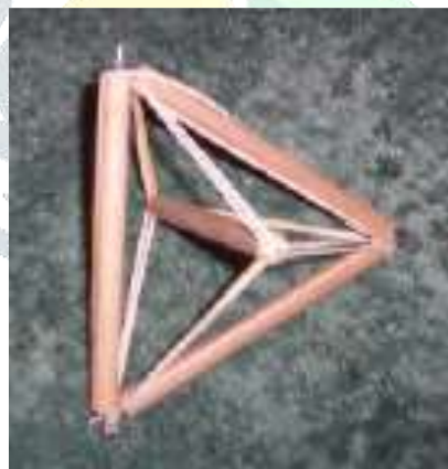
fig:1 false tensegrity
