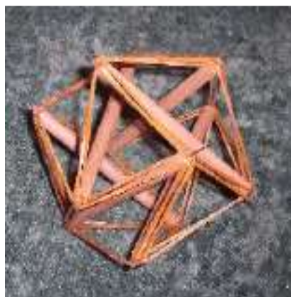
fig:2 pure tensegrity
