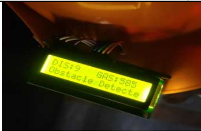
Fig-5: Results of ultrasonic sensor on LCD display
