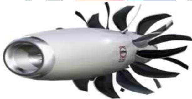
Fig: Counter Rotating open rotor engine
