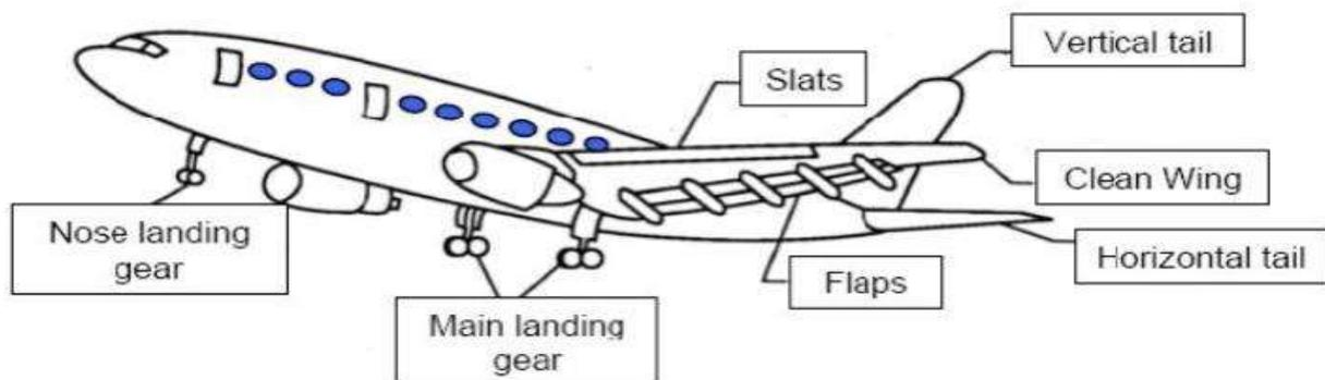
Fig2: Sources of Airframe Noise
