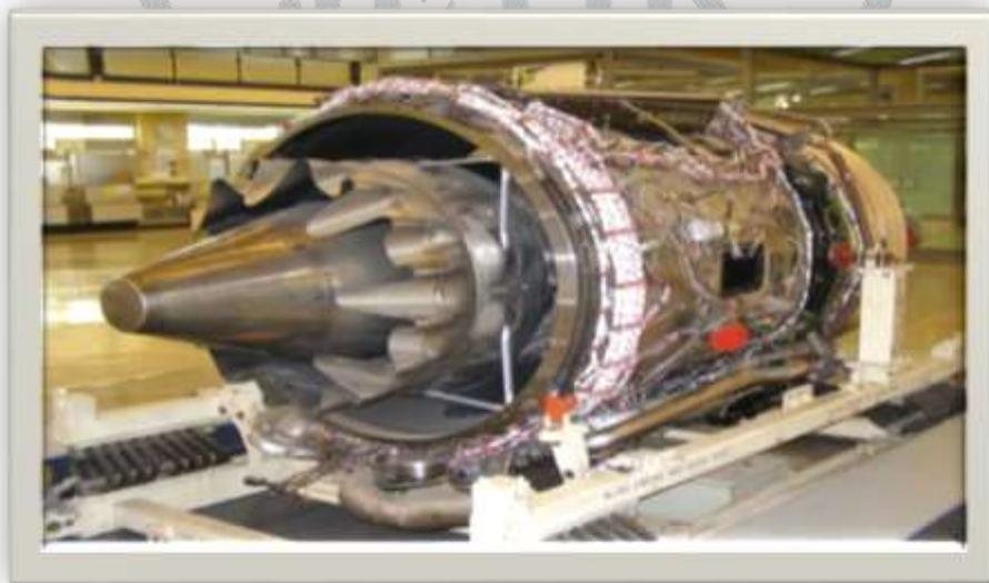
Fig3: Rolls Royce BR700 Engine with Forced Mixer.
