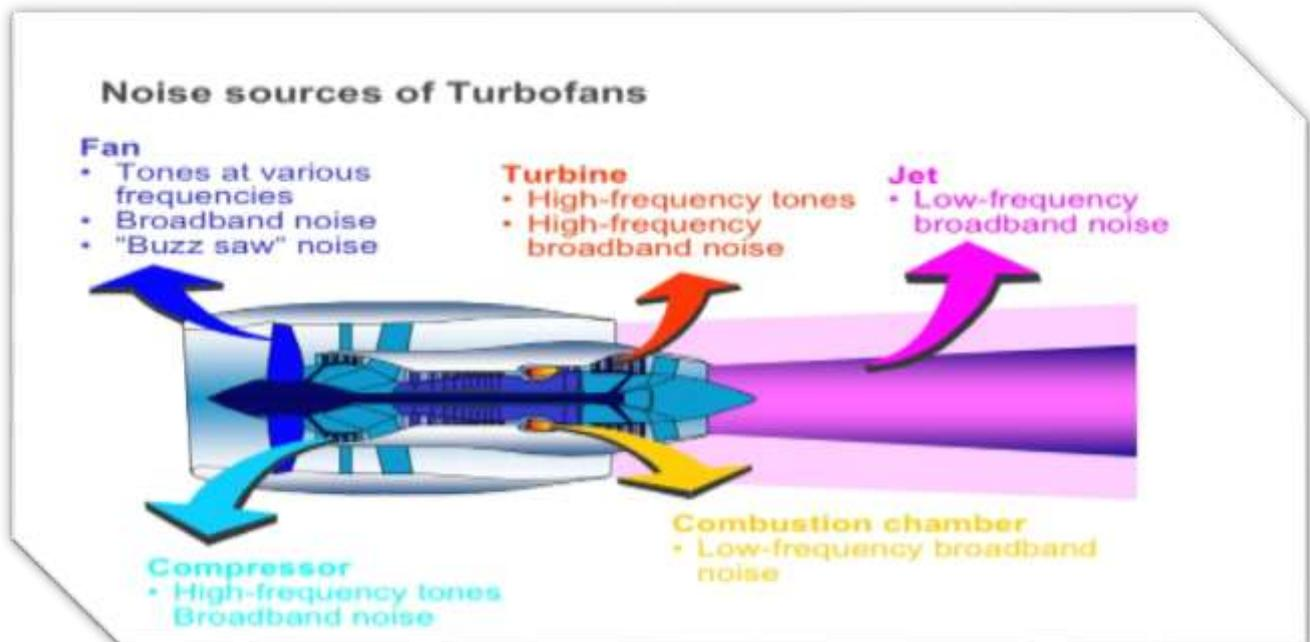
Fig1: Noise Sources of Turbofans
