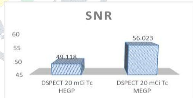
Figure 11. Relation between collimator type of DSPECT & SNR
