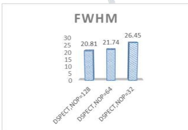
Figure 12. Relation between number of projections of DSPECT & FWHM.
