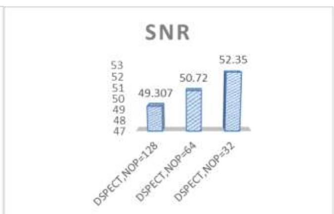
Figure 15. Relation between number of projections of DSPECT & SNR.
