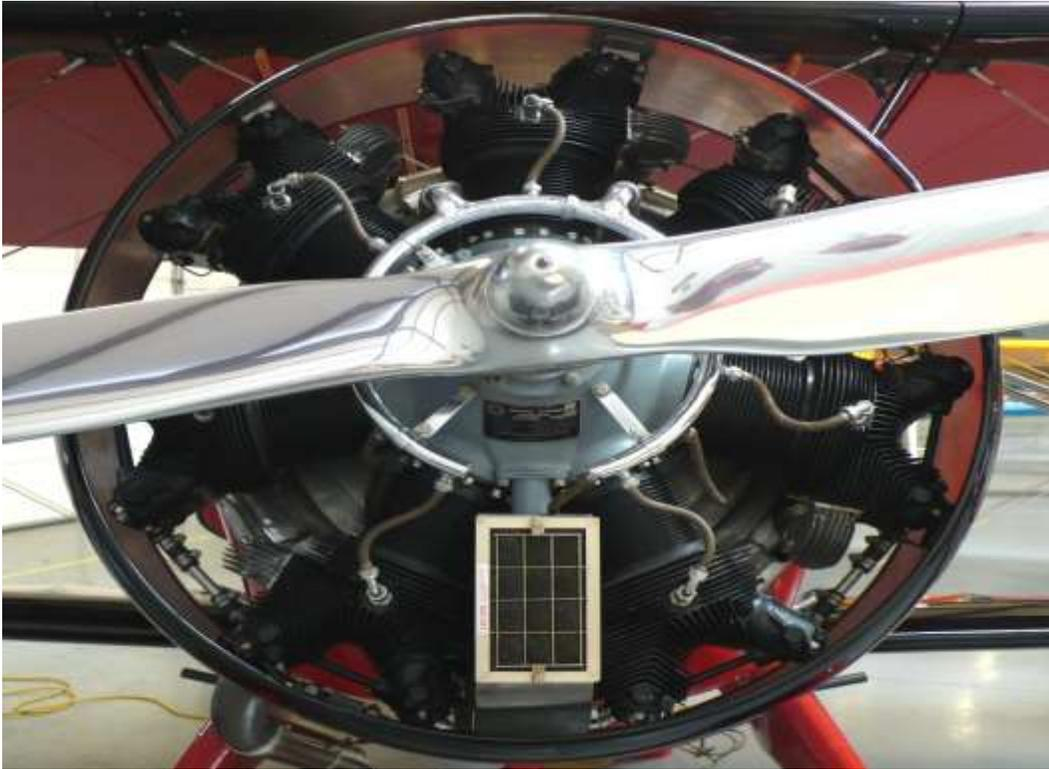
***Radial engine is type of “Internal Combustion” engine .It is used in an aircrafts and most of the flying vehicles. It have a lot of cylinders in an odd number series and all are connected in a one crankshaft in a radial position using connecting rod .***
