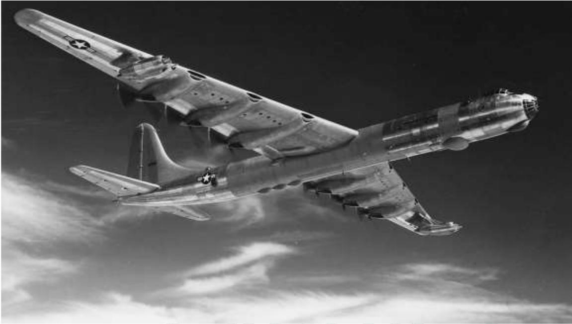
*To get more power out of a radial engine, engineers added multiple rows of cylinders. The Pratt & Whitney Wasp Major uses four rows of seven cylinders (that's 28 total cylinders!) with a supercharger to generate up to 4,300 horsepower. It powered many of the last piston-powered large aircraft, including the B-36 Peacemaker (which used six Wasp Majors and four turbojets) and the Martin Mars.*
