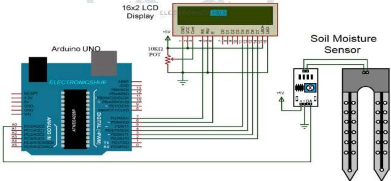
FIGURE: - 7 Circuit Diagram
