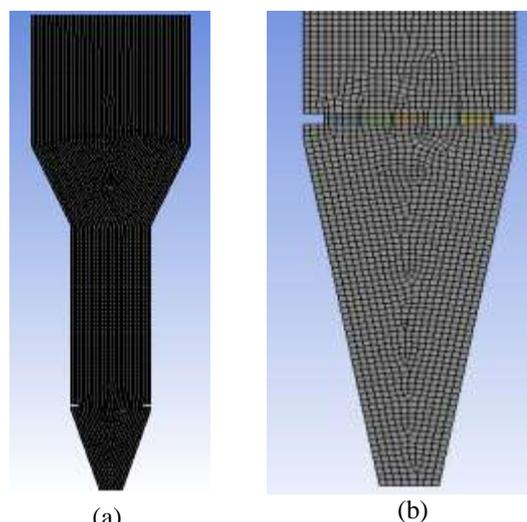
(a) (b) Fig. 11 Mesh geometry and Closer View[30]
