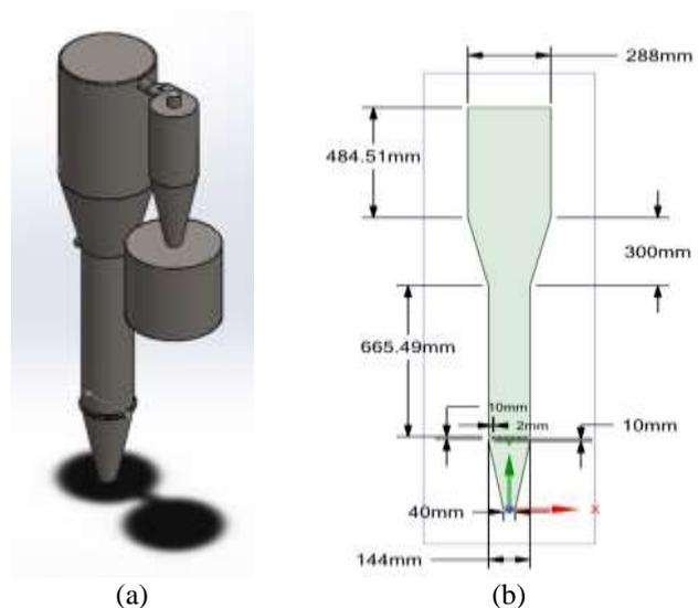
(a) (b) Fig. 10 Designed CAD BFBG Model[30]
