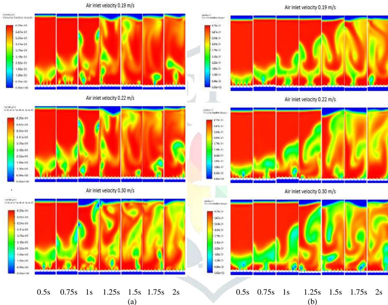
Fig 12. Volume fraction distribution for (a) the Sand (b) Face Mask Particles using the Syamlal and O'Brien drag model with three inlet velocities 0.19 m/s, 0.22 m/s and 0.30 m/s [30]
