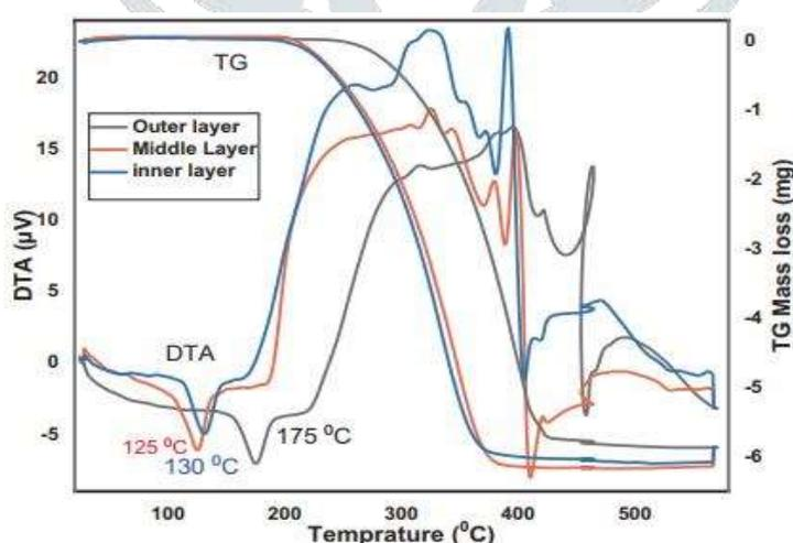
Fig. 5 GA/differential thermal analysis of the three layers surgical face mask [13]
