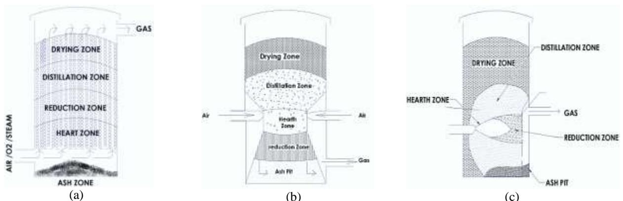
Fig. 7 shows (a) Updraft (b) Down Draft (c) Crossdraft types Fixed Bed Gasifier [22]
