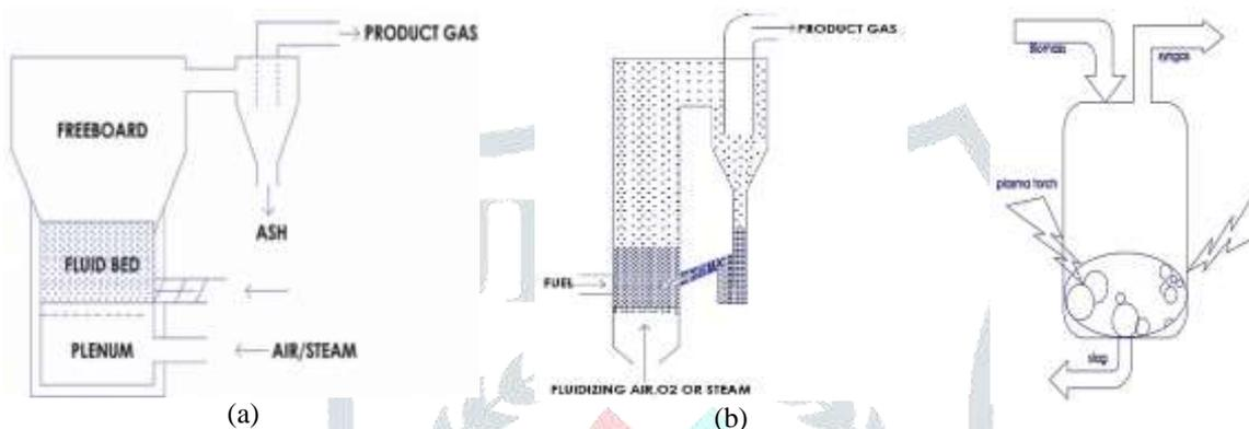
Fig. 8 schematic diagram of (a) BFB gasifier (b)CFB gasifier [22]
