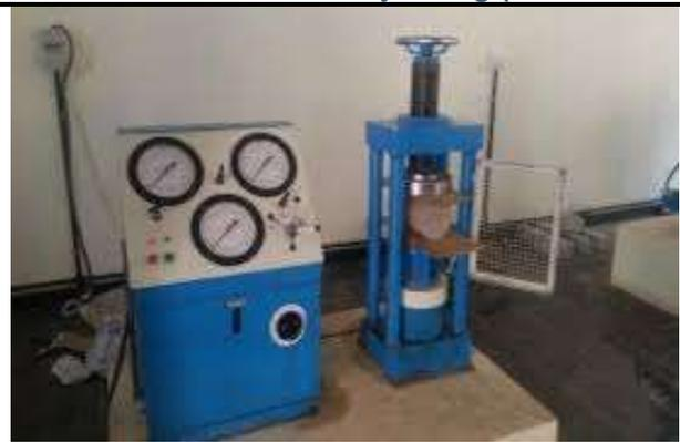
**Fig 6. Split tensil strength testing**
