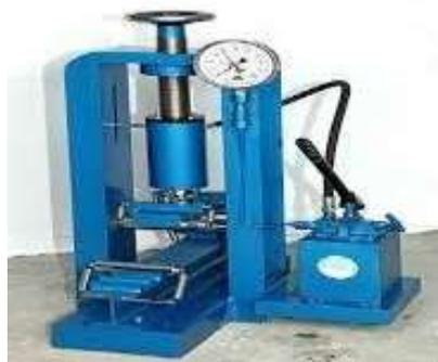
**Fig 7. Flexural Strength Testing**
