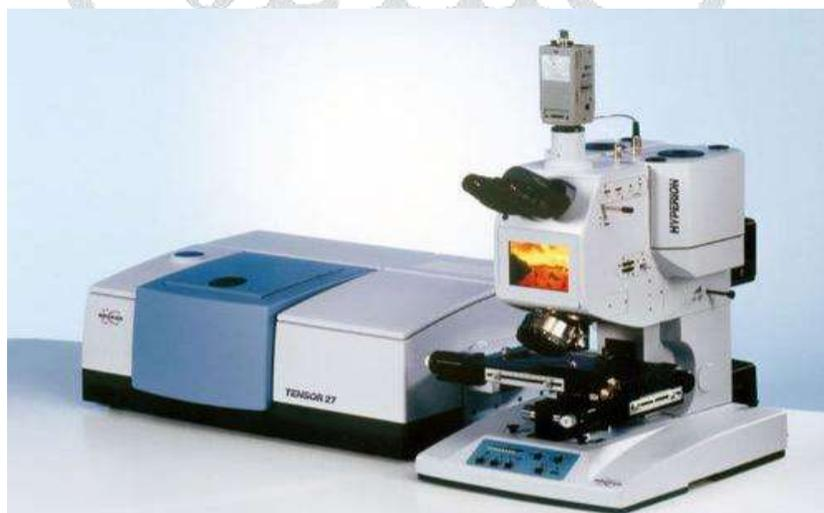
Fig.3: Fourier transform infrared spectroscopy
