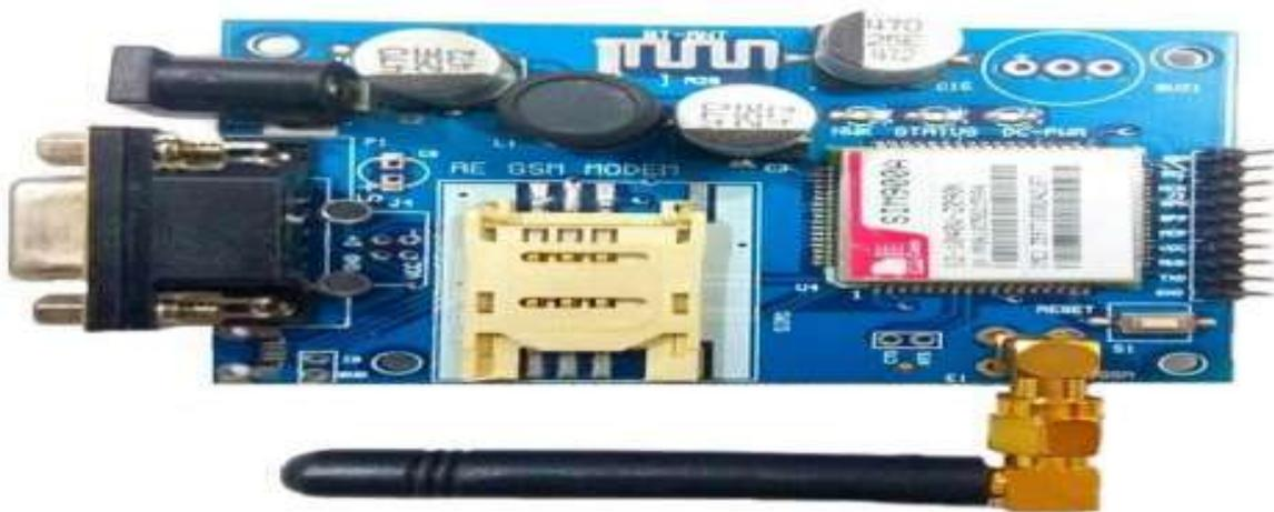
Fig 4:-SIM 900A GSM MODULE
