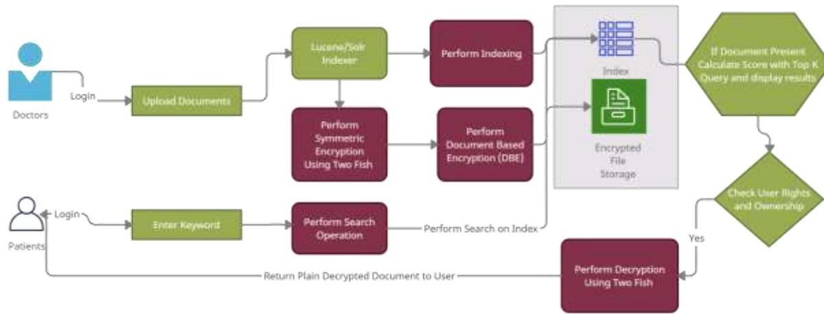
Figure 1.0 Proposed Architectural Flow Diagram
