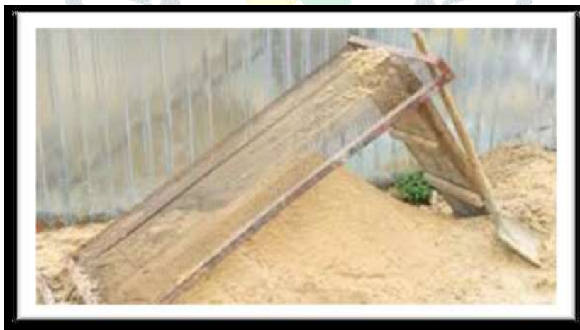
Figure 2.1 Traditional sand filter
