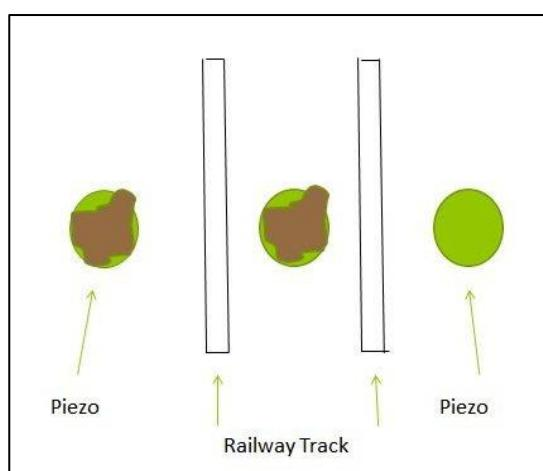
In this case also, any 2 sensors will give a high (including the middle one) and the most important thing is that there will be very less or no delay between them. So, the Wi-Fi module will send the GPS co-ordinates as well as a message – “Landslide” to the database.
