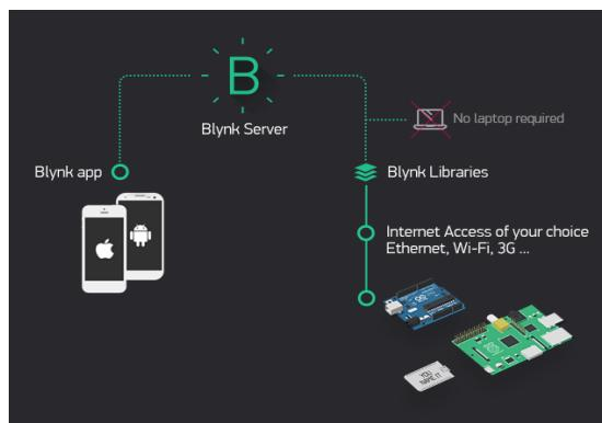
**1. Blynk App** – It provides us various widgets to visualize the data send by the microprocessor. Here we have used the Google map view to display the GPS coordinate of the place where landslide or Animal is detected.
