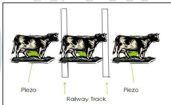
In this case, all the 3 sensors will give a high but there will be considerable delay between the High given by the sensors. The micro-controller will sense this and the Wi-Fi module will send the GPS co-ordinates and a message – “Animal Passed” to the database.
