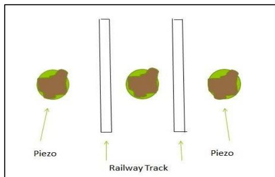
During this condition, all the sensors will give a high and there will be very less or no delay between them giving a high. The microcontroller senses this and sends the GPS co-ordinates of the sensor along with a message – “Landslide”, to the database on the local server.
