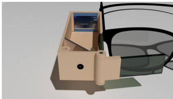
Fig:24 (b) Mounting of all hardware inside the case.
