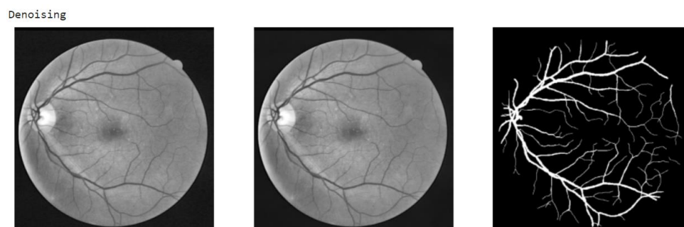
Fig.10. Fast cv2 Denoising of gamma corrected images
